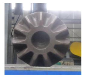
Fig. 11. Forged bevel gear
