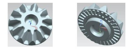
Fig. 2. Forged bevel gear
