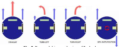
Fig. 2. Proposed drive mechanism of 2 wheels
