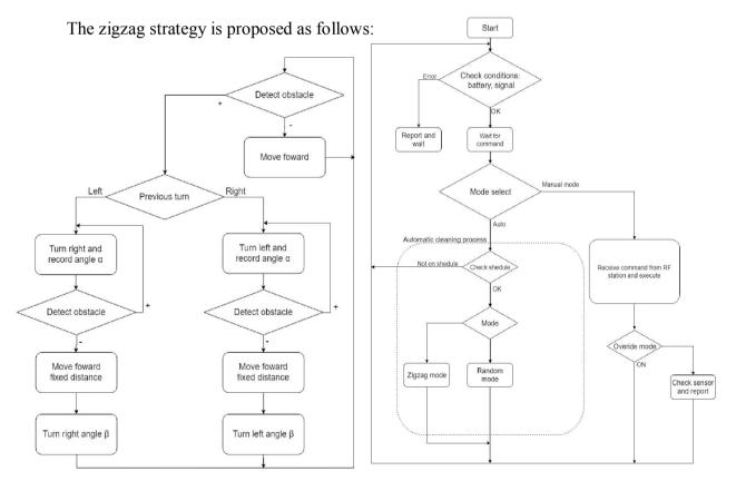
Fig. 9. The diagram of proposed zigzag movement control algorithm
