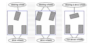
Fig 1. Several common driving mechanism
