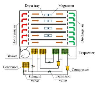
Fig. 1. Schematic diagram of the combined heat pump - microwave dryer used in this study
