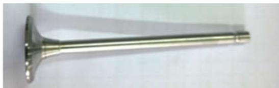
Figure 9. An sample of fabricated intake valves
